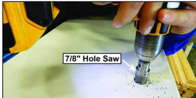
Figure 3: Drilling the Initial Hole
